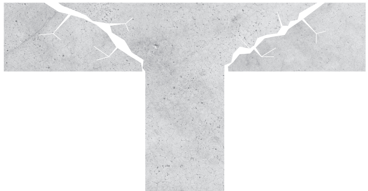
Example of Failure due to punching shear
