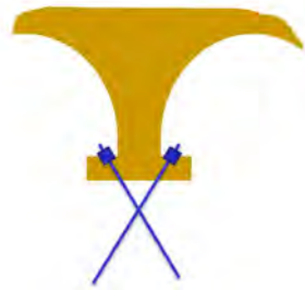
Bridge and building Mini Piles
