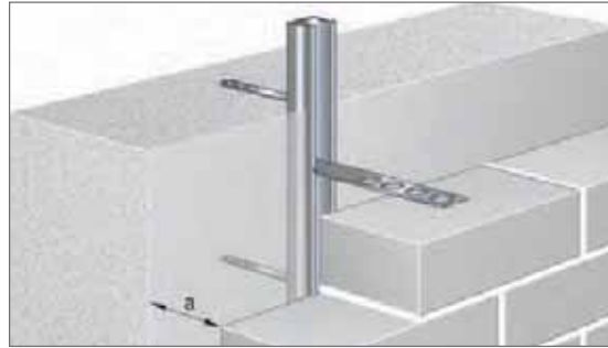
Connection of brickwork support shells to reinforced concrete components with brick tie channel Kt 28/15-D and anchor.
